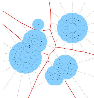
**Figure 2:** The pathway diagram (bold line) of a collection same-size discs that approximate the discs depicted in Figure 1. The discarded portions of the Voronoi diagram of their centers is depicted using dotted lines.
