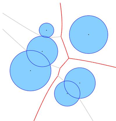
**Figure 1:** The pathway axis of a collection of discs (bold line). The discarded portions of the medial axis are colored gray.
