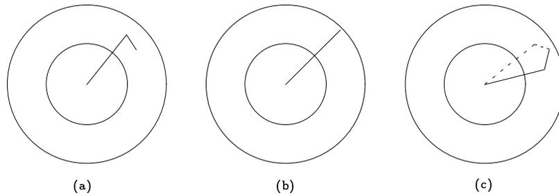
Figure 7: The kinematics of the two-link arm
