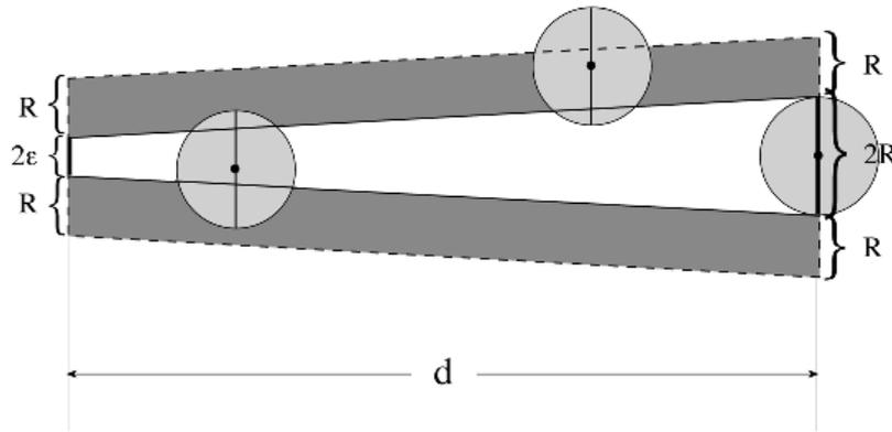
**Figure 3:** A sphere is (partially) occluding the sphere on the right from  $C_\epsilon$  (the  $2\epsilon$  segment on the left)  $\iff$  it intersects with the smaller trapezoid  $\iff$  its center lies within the larger trapezoid. Here, only the left sphere is a strong occluder.
