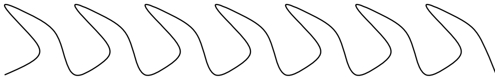
Figure 6.2: A one dimensional illustration of a swept volume, where the xy -partitioning process results in many terrains and therefore many connectors.
